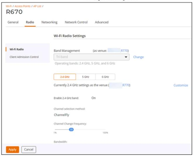
4. (Optional) For **Band Management**, the default setting is to use the band operation mode of the venue (the field is inactive and grayed out). To customize the band operation mode at the AP level, click the **Change** option; the field becomes active, allowing you to modify the setting. For more information, refer to *Switchable Radio Frequency Support (GUID-3E0112D7-A87A-49BE-874A-75EB6A5B3481.html)*.
